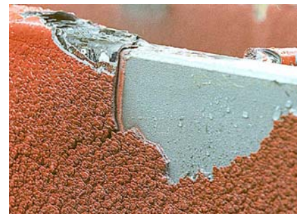
Over spray removal from skids
